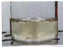
Figure 3. Visible aggregates formation of infliximab biosimilar within a vial when stored over 6 months after sterile compounding.
